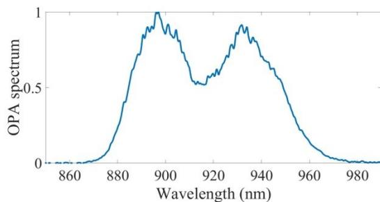
Fig. 4 - An optimized spectral output obtained with non-collinear optimization of the dual stage LBO. The two gain peaks are equivalent to the optimum phase matching for each one of the crystals.
