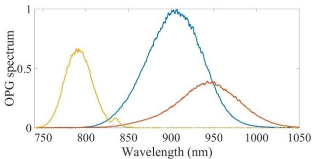
Fig. 3- 3 OPG spectra, centered at 790, 910 and 950nm obtained by changing the phase matching angle.
