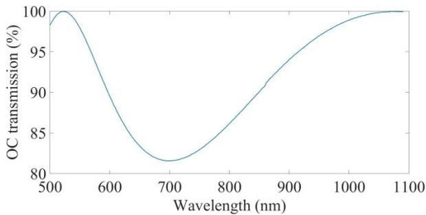
Fig. 2 - Output coupler transmission profile
